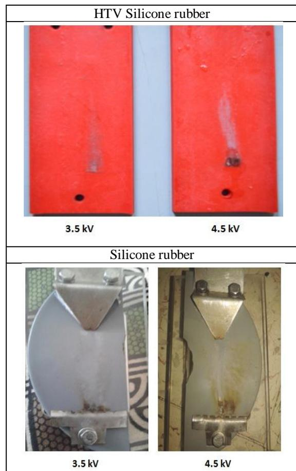
Figure 9 Visual appearance of sample at end of tests
